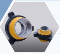
FLUXO Hammer Unions are made from Forged Alloy Steel. The steel has High Anti Corrosive property and High Strength. It comes with Weldon and Threaded type with all size from 1" to 12". From Sch 40 to 160 and in XXH type also. FLUXO Hammer Unions cover the Working Pressure range from 100 PSI to 20000 PSI. We provide all Sour Services Hammer Unions with Viton Seal Rings.
